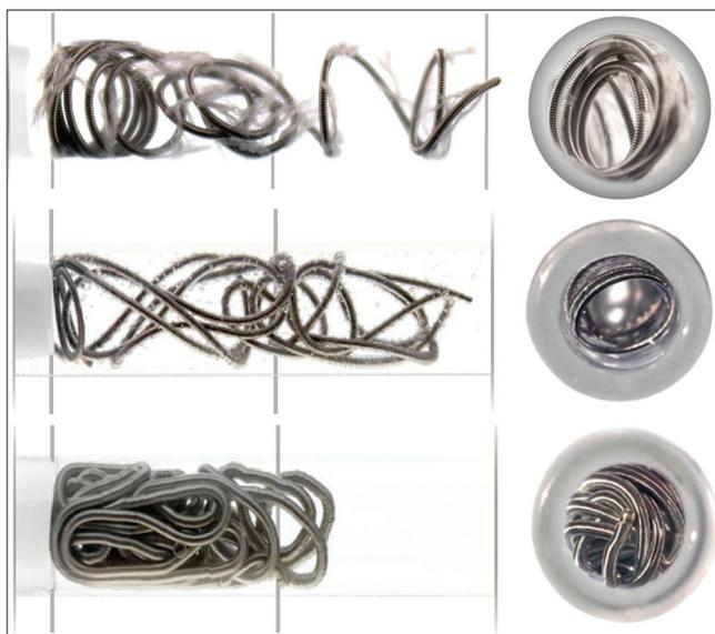
**Figure 2:** Lateral and vessel cross-sectional images in equal size glass vessels of fibered, hydrogel coated, and soft bare-platinum Ruby Coils. Top: Fibered coil; Middle; hydrogel coil Bottom; soft, bare-platinum ruby coil. Ruby coils have thicker and softer coil loops that densely pack creating a mechanical occlusion with less reliance on thrombus formation. Images supplied by Penumbra Inc.
