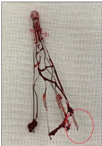
Figure 4: Greenfield filter post-removal. Recurved strut hook shown inside the circle.
