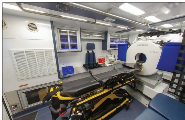
Figure 1: A standard interior of a mobile stroke unit. Note the presence of standard ambulance equipment, a computed tomography scanner, and point-of-care laboratory equipment. Photo courtesy of Frazer, Ltd.
